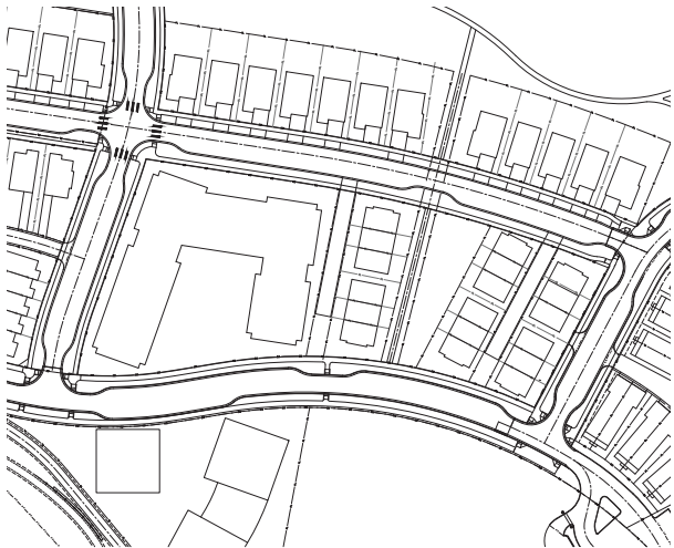
3. Mixed use / multiple family with street level retail at SW corner (parking within building) and cottages on east half.
