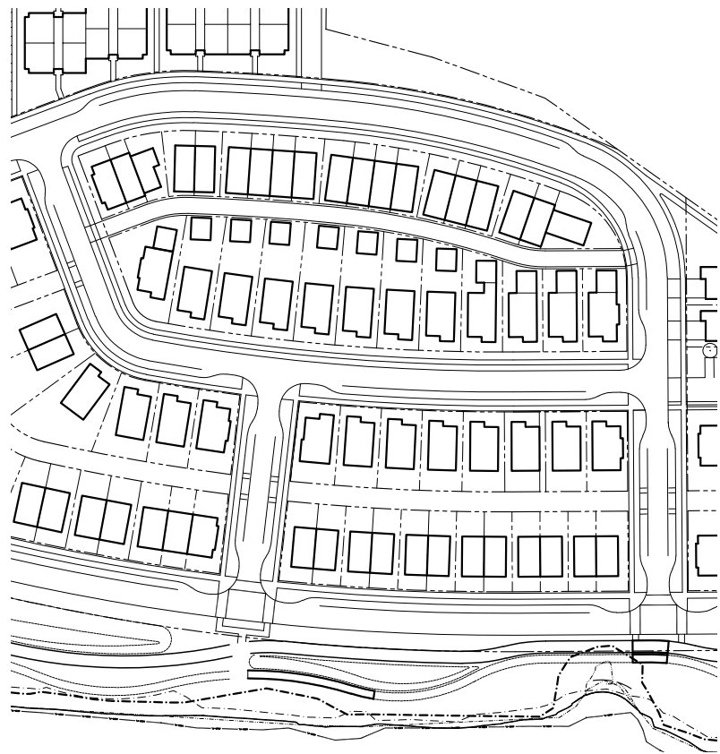
2. Alley option provides an opportunity for rear-loaded single family homes and rear-loaded townhouses that take advantage of sloped topography to have garages below the main level of the units.
